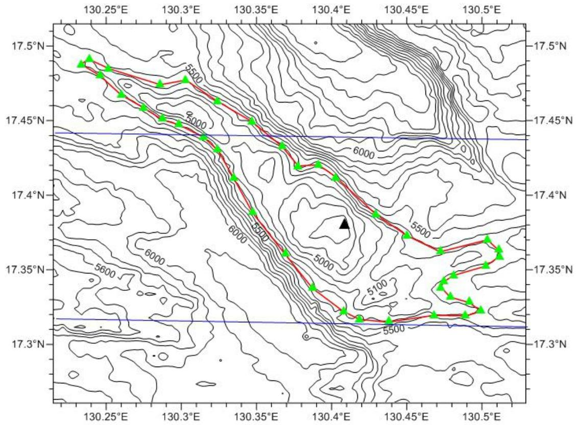
Fig.4 Bathymetric map of the Jixia Hill, showing track lines.
