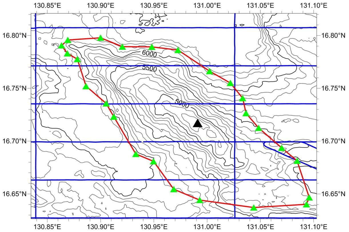
Fig.4 Bathymetric map of Jiayue Seamount overlain with track lines (Contours are in 100m, blue lines for the track lines)
