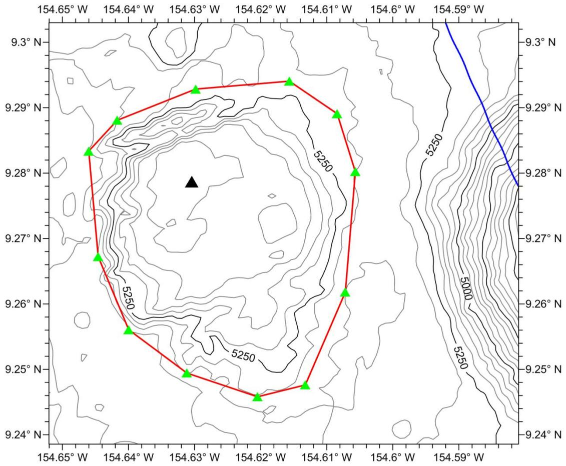
Fig.4 Tianxian Hillisobath line and survey line map (the isobath line spacing is 50m, the blue line is the survey line)
