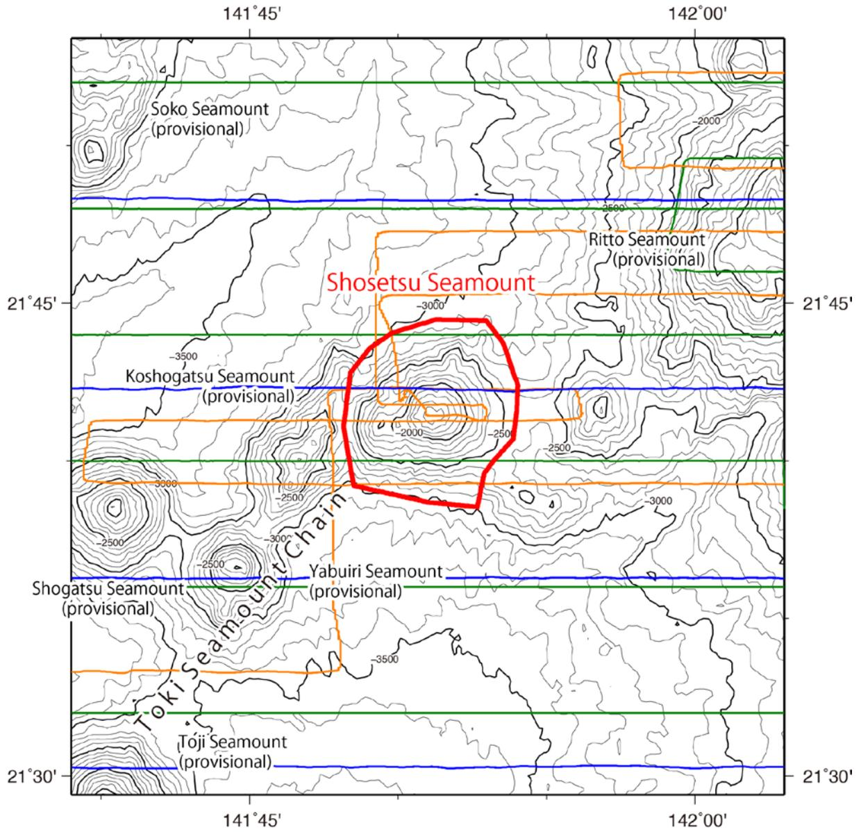
Fig. 2. Bathymetric map of the Shosetsu Seamount, shown with track lines. Contours are in 100 m.
