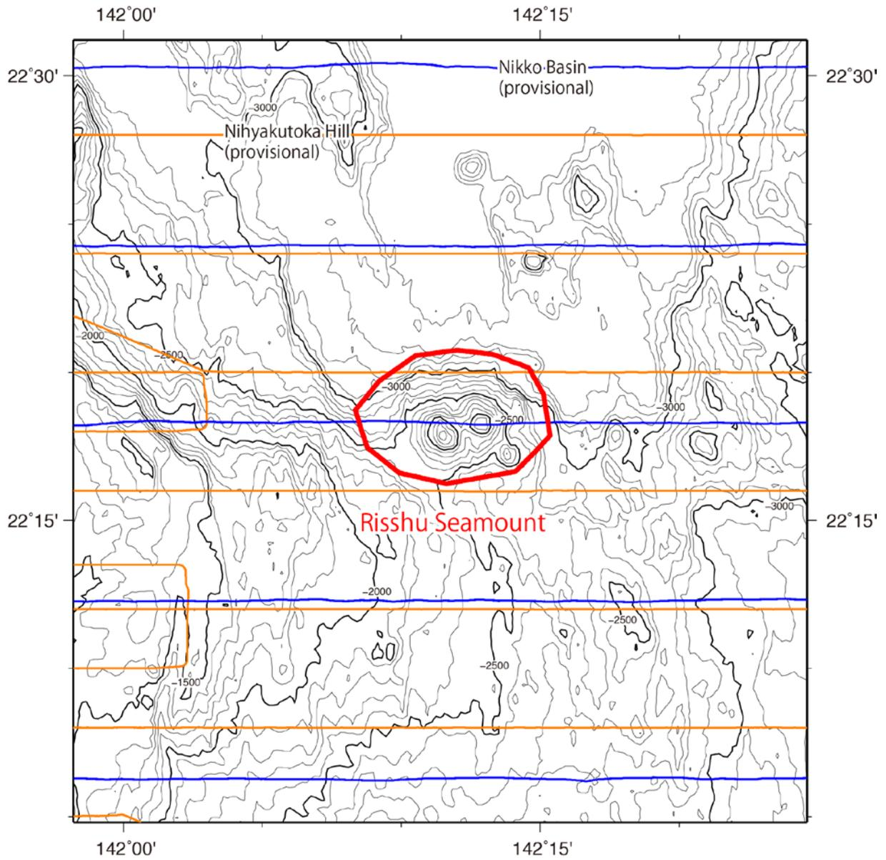
Fig. 2. Bathymetric map of the Rishu Seamount, shown with track lines. Contours are in 100 m.
