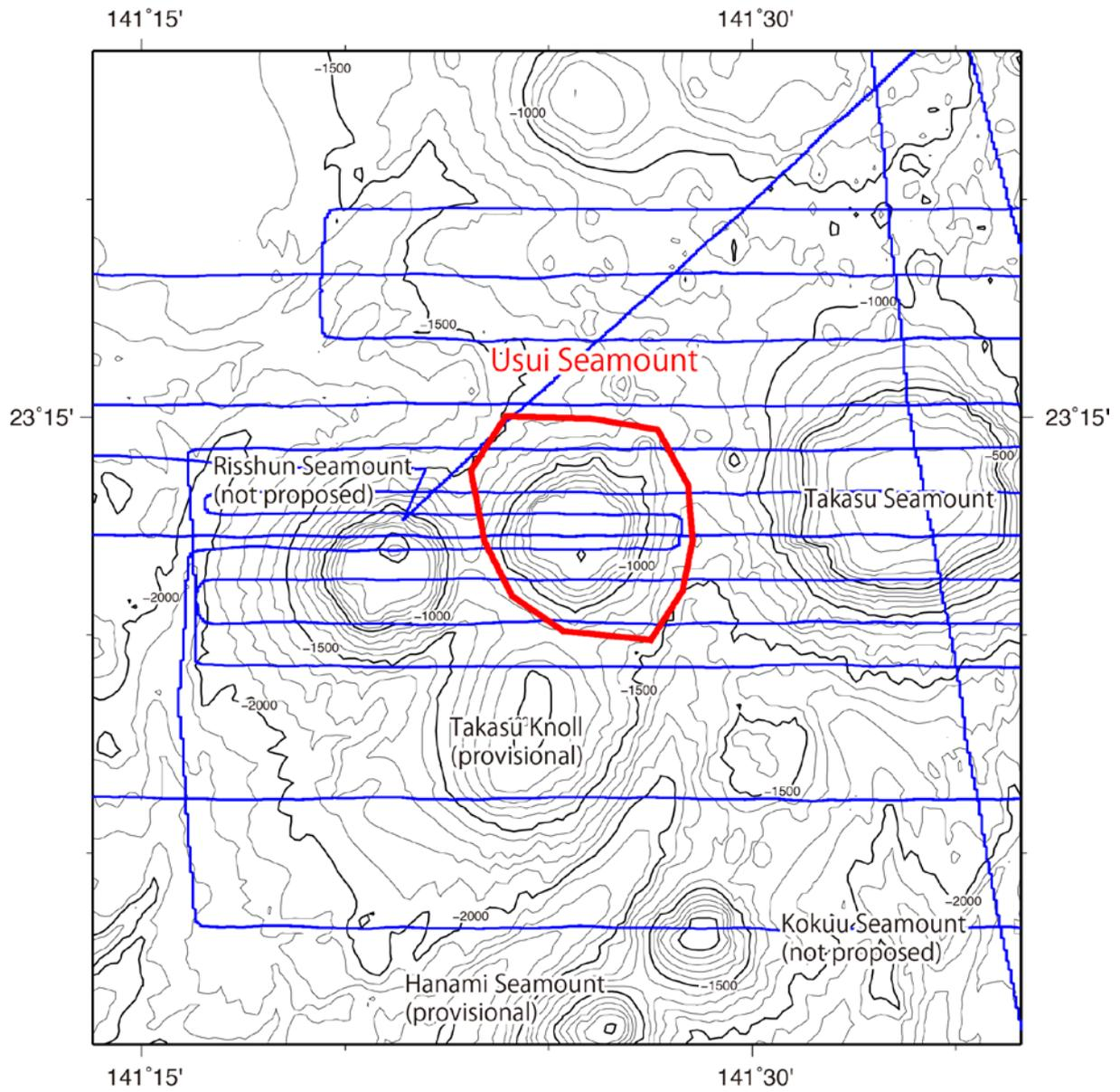
Fig. 2. Bathymetric map of the Usui Seamount, shown with track lines. Contours are in 100 m.
