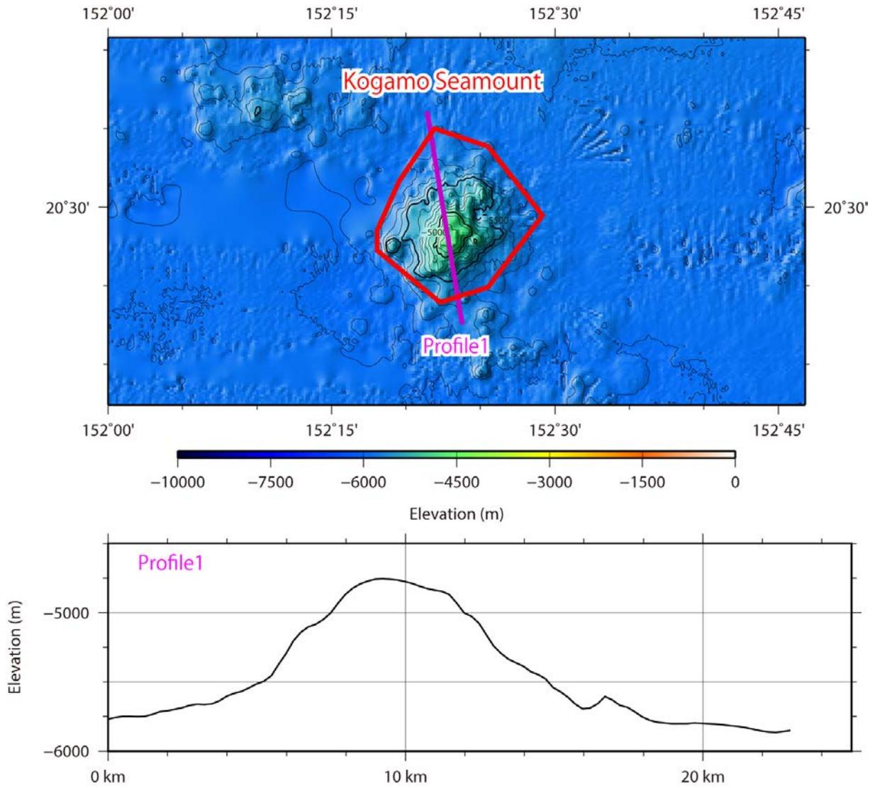
Fig. 3. Bathymetric profile across the Kogamo Seamount.
