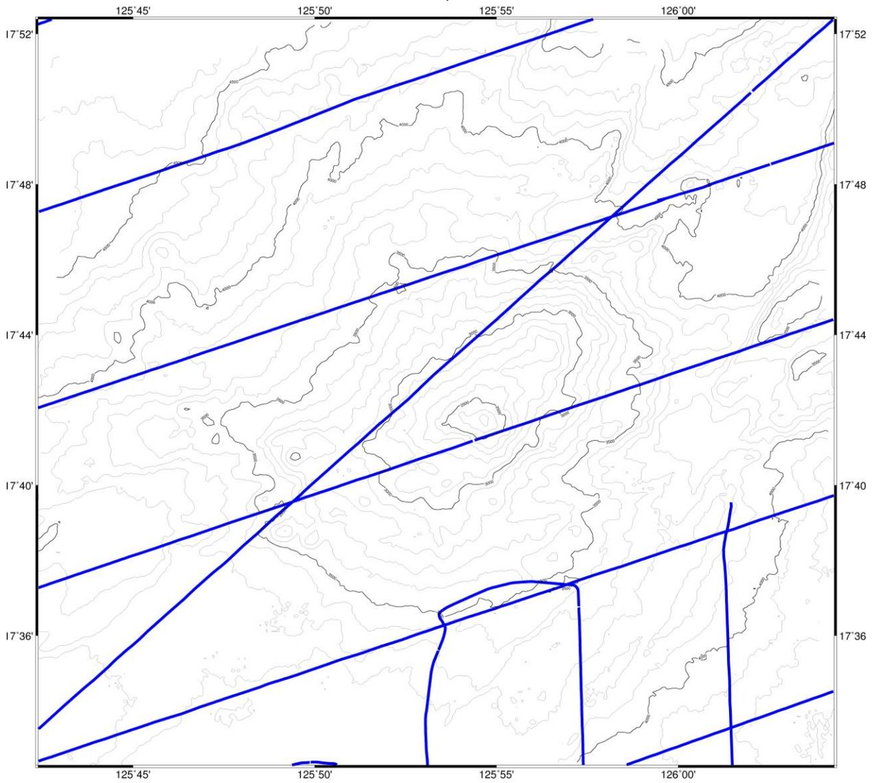
Figure 3. Bathymetric map of Toog Seamount showing track lines.
