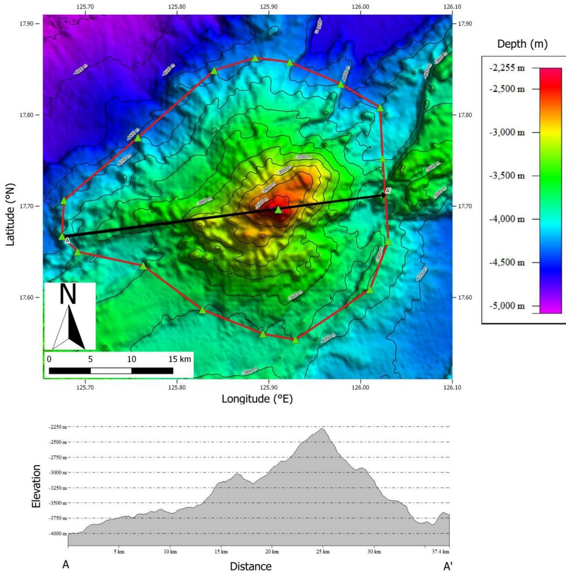
Figure 7. Profile of the Toog Seamount from the south to the north edge (A – A')
