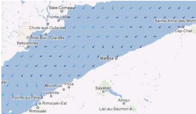
Figure 1 - An Example of a Gridded Coverage of Surface Currents in the St. Lawrence River (High Tide - Reverse Flow)
