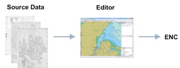
Figure 8. The traditional method of ENC production involves the compilation of individual ENCs from source data. There is no database and the ENC functions as both product and data repository.
