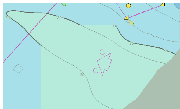
Figure 4. The northern ENC has the 15m contour omitted. This results in a broken and disjointed safety contour.
