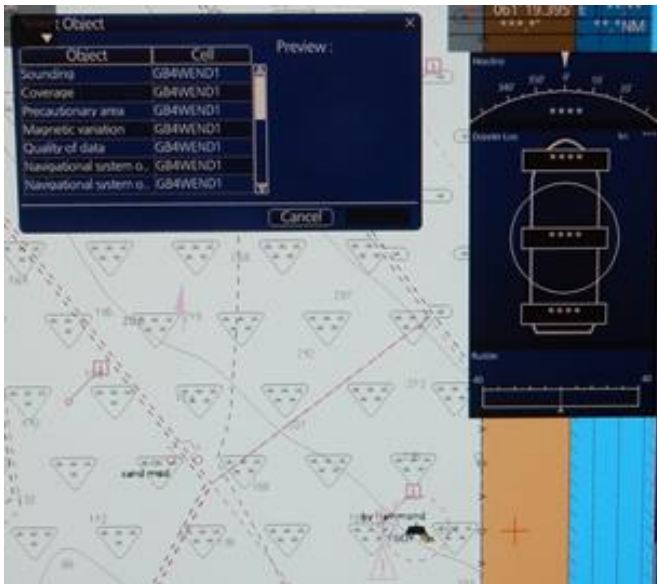
Figure 20 – ECDIS D GB4WEND1 displaying at 45k with PILBOP no longer visible
