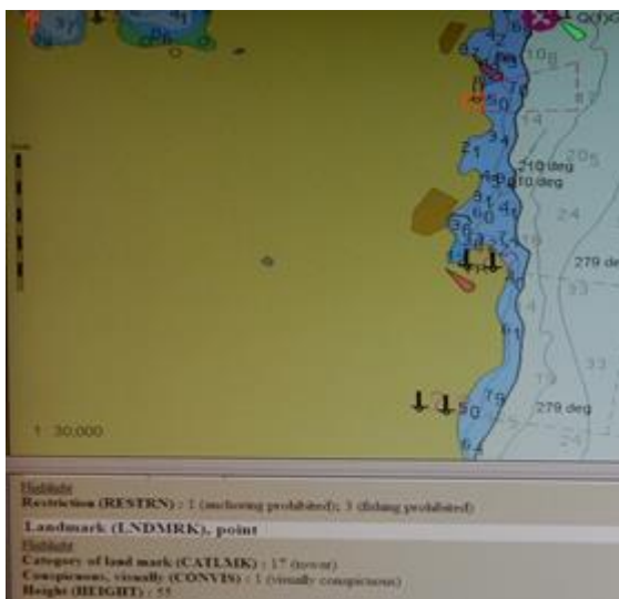
Figure A10 – LNDMRK (convis) displaying on GB4WEND3
