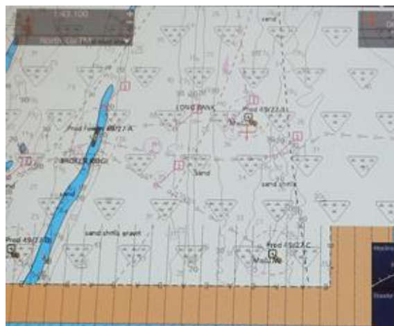
Figure D9 – Both cells displaying overlap at 43k
