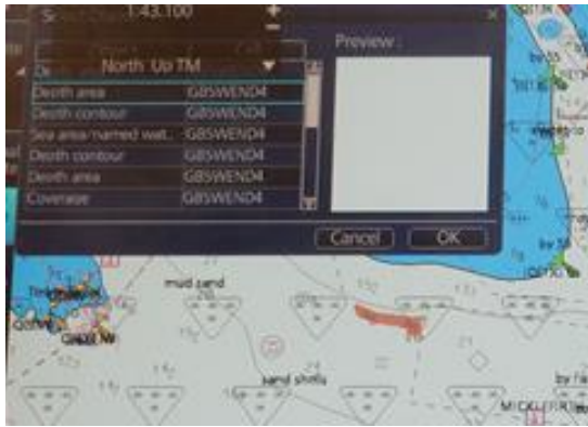
Figure D19 – Shoal depth displaying on GB5WEND4
