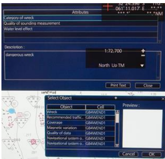
Figure D17 – ECDIS D displaying GB4WEND1 WRECKS with dangerous wreck attribution
