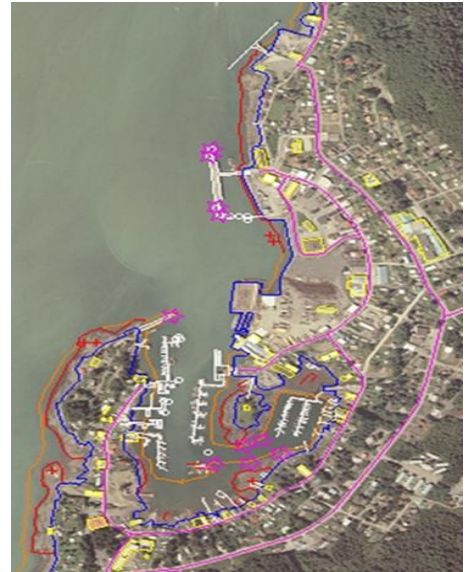
Wrangell, Alaska. Features added include Mean High Water, Mean Low Water, obstructions, dangers, and aids to navigation.
