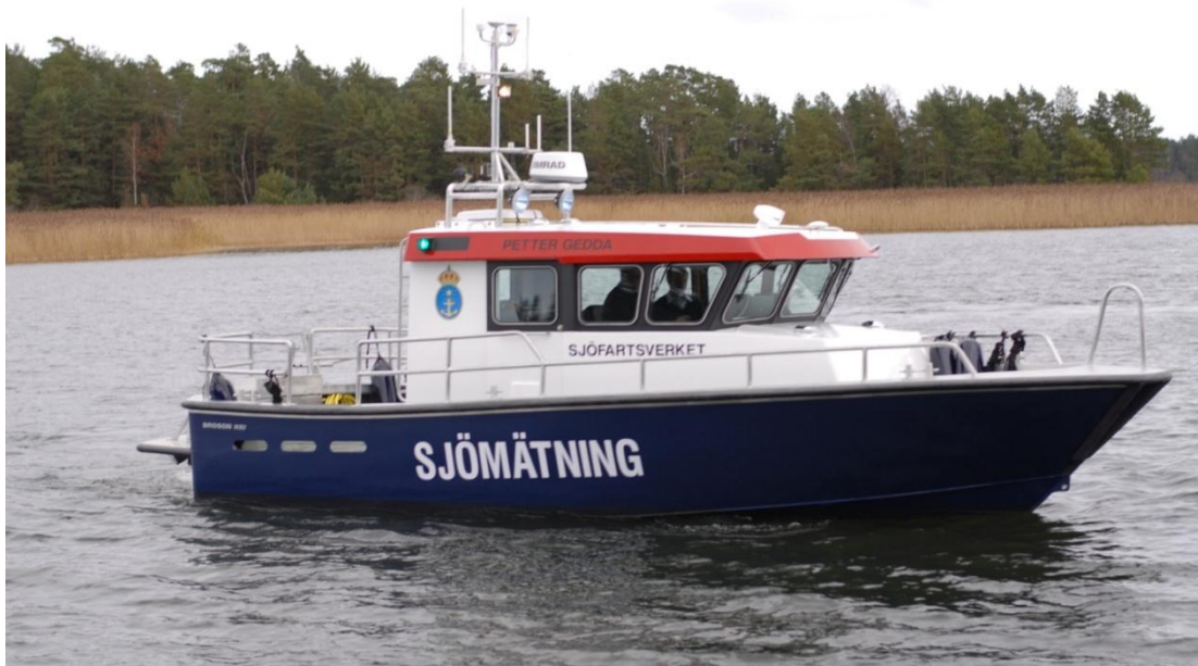
PETTER GEDDA , a 8.5m boat built for near shore and port jobs. Equipped with RESON 7125 multibeam echo sounder.
