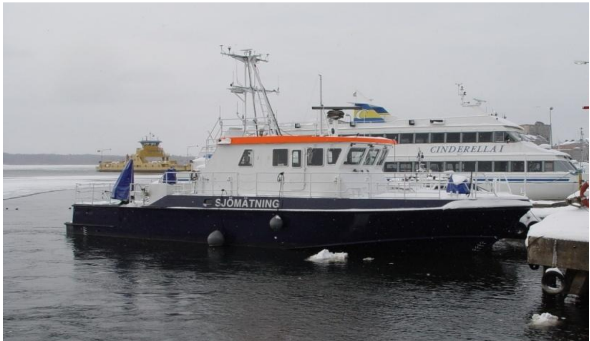
JOHAN MÅNSSON a 20m boat equipped with RESON 7125 multi-beam echo sounder for work in the archipelago. The crew is 3-4 persons with two work places for post processing.
