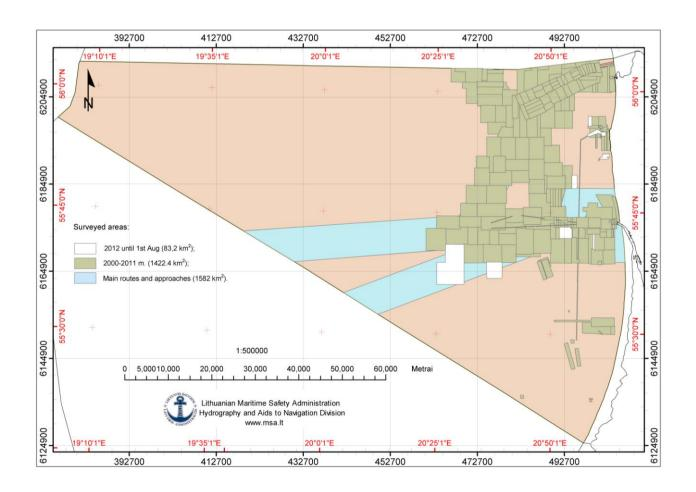
The area of main routes and approaches is **1582** km<sup>2</sup>. Up to August 2012 the area of **1065** km<sup>2</sup> of main routes and approaches was surveyed. In **2012** until 1st August there were surveyed **83** km<sup>2</sup> (see fig.).
