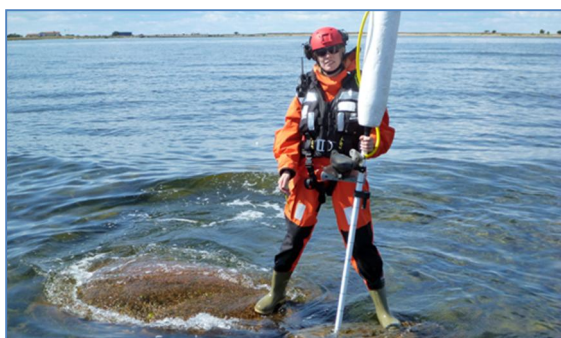
Fig 15 Surveying a rock awash outside Öland in August 2012.
