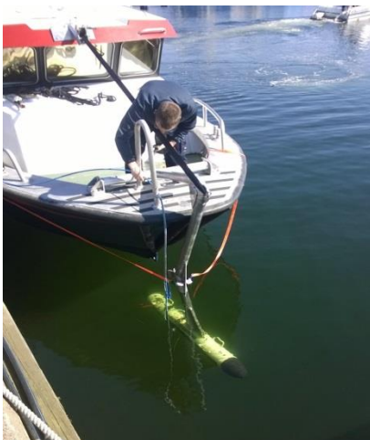
SMA vessel Petter Gedda during test fitting of the SMA Klein 5000-Bathy
