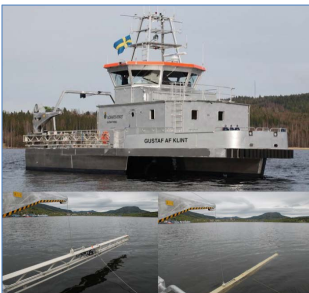
Figure 3 Bar sweeping survey vessel Gustaf af Klint. The bar is transverse across the stern and is here submerged into the water.
