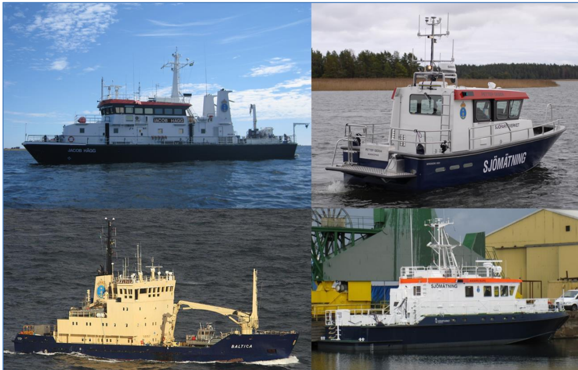
Figure 4- SMA Survey vessels equipped with multibeam. To the left the two survey vessels Jacob Hägg and Baltica where surveying is performed 24 hours per day and 7 days per week, weather permitted. To the right the two survey boats Petter Gedda and Anders Bure.
