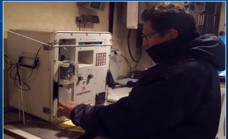
Salinity measurement in Guildline salinometer
