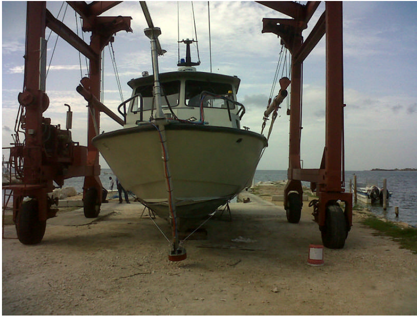
Coastguard launch rigged with Kongsberg EM3002 MBES
