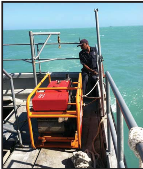
Generator Placement & Hand SSS Towing present safety hazards to BPA hydrographic personnel.
