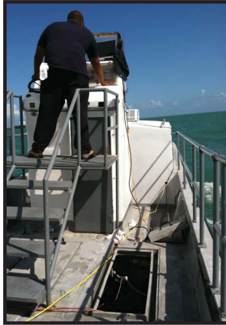
Engine Compartment Hatches are left open during vessel operation.
