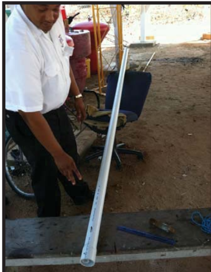
Mounting the Valeport 740 Tide Gage – Fixed to a 1-inch PVC pipe, the sensor was mounted inside a protective 3-inch PVC pipe well (left). BPA personnel strapped the well to a concrete piling near the PBL pier (right) and manually measured the distance between the sensor and top of the well to provide a leveling point to the benchmark.
