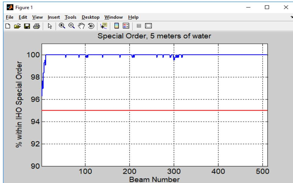
Surface statistics were generated using the CARIS “QC Report ...” and “Compute Statistics...” CSAR surface tools. The  $2\sigma$  standard deviations of the grid points for all surfaces were within IHO order 1a. The results indicated that 100% of the bathymetric surface met IHO order 1b.
