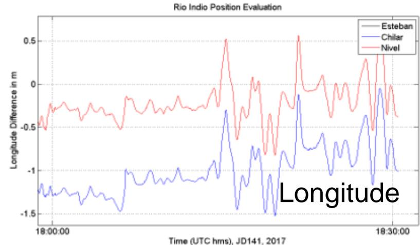
Latitude and longitude difference results for the boat while stationary in Santa Rosa. Results show that the horizontal positioning meets the requirements for IHO order 1b (5m).
