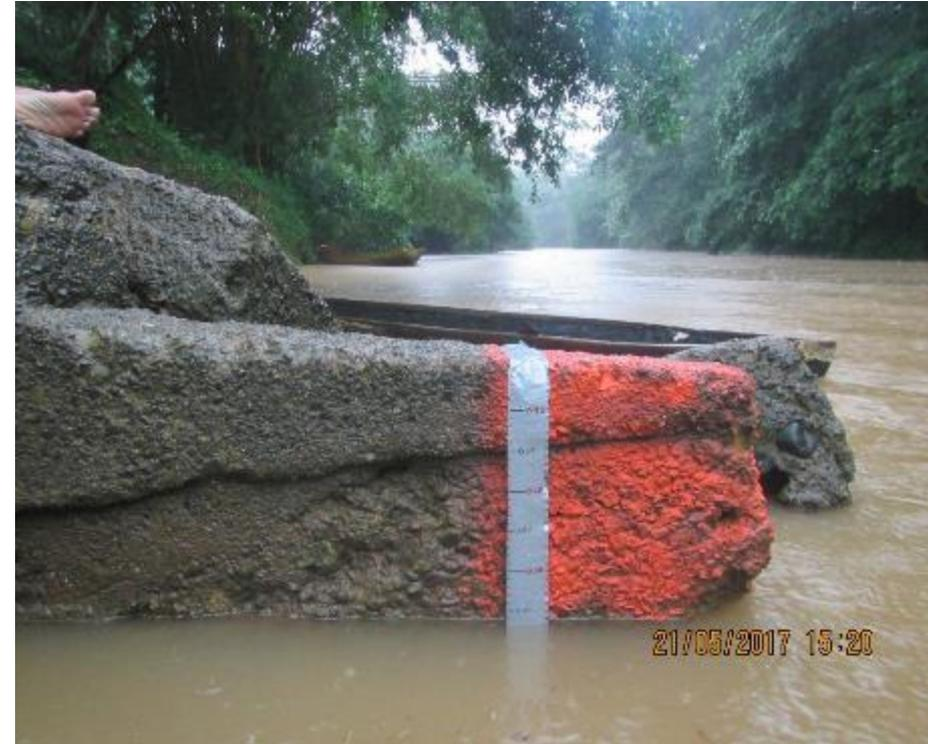
Water level measured relative to spray painted concrete slab. Used duct tape with graduations for tide staff. Water went from 0.4 m below to level in 20 minutes, then to 1.5 m above in another 30 minutes. This occurred after a significant rain event
