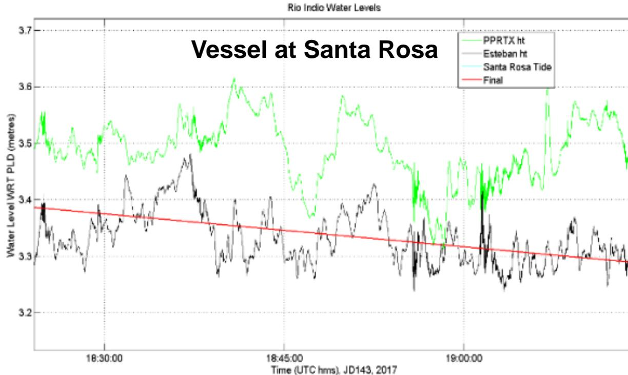
Plot of heights, relative to PLD, while the boat is stationary in Santa Rosa. **The Nivel GNSS heights are in good agreement with the measured water level.**
