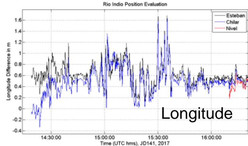
The comparison at Chilar, with the boat stationary. Plots are in metres and are the result of differencing the single baseline solutions from the PP-RTX solution.
