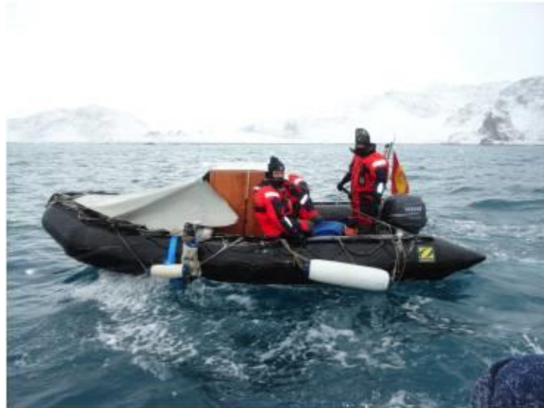
Figure 7. Very shallow water bathymetry system operated from a small rubber boat in Antarctic area
