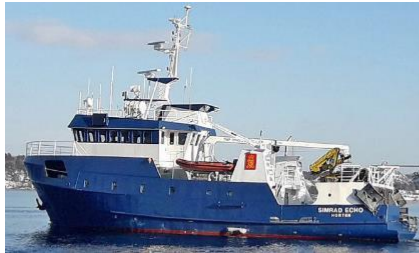
Simrad Echo used as «USV». MBR 179 installed together with HIPAP for coms with Hugin
