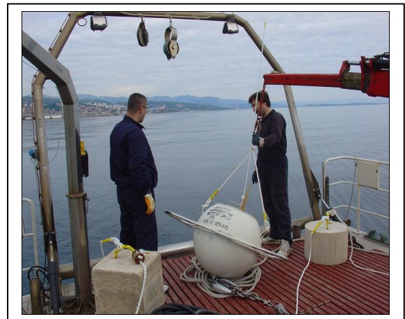
Fig. 9. Deployment of waverider buoy on 6 May 2009
