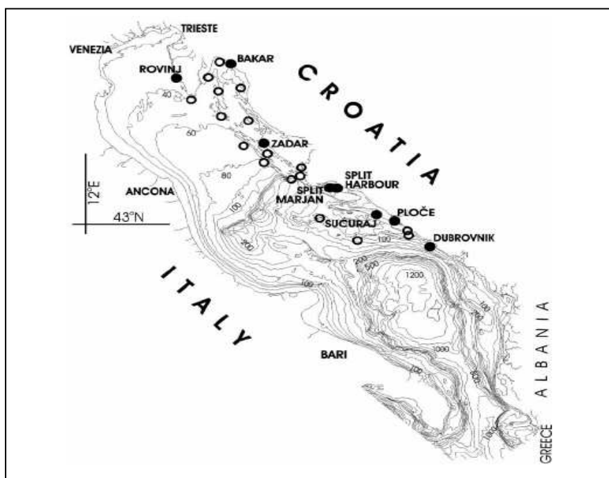
Figure 6. Schematic Adriatic Sea map with tide gauges operational in 2007-2009 (filled circles) and the last 50 years (blank circles) along the Croatian coast of Adriatic Sea.
