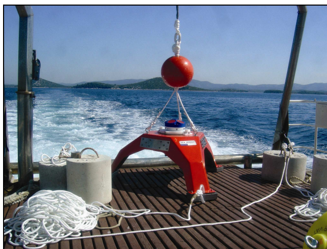
Figure 18. Acoustic Doppler Current Profiler ready for deployment, aboard RV “Hidra”
