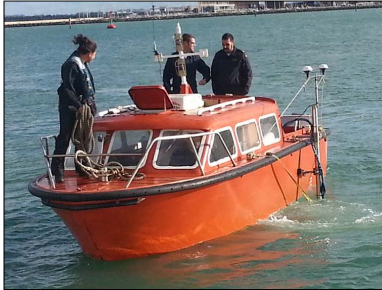
Figure 4. Very shallow water bathymetry system operated from a boat
