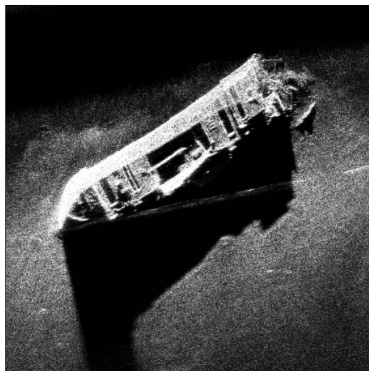
Figure 7. Wreck image obtained with the synthetic aperture sonar
