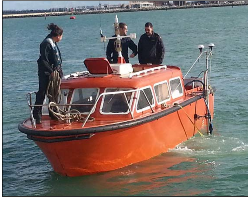
Figure 4. Very shallow water PDBS operated from a boat.
