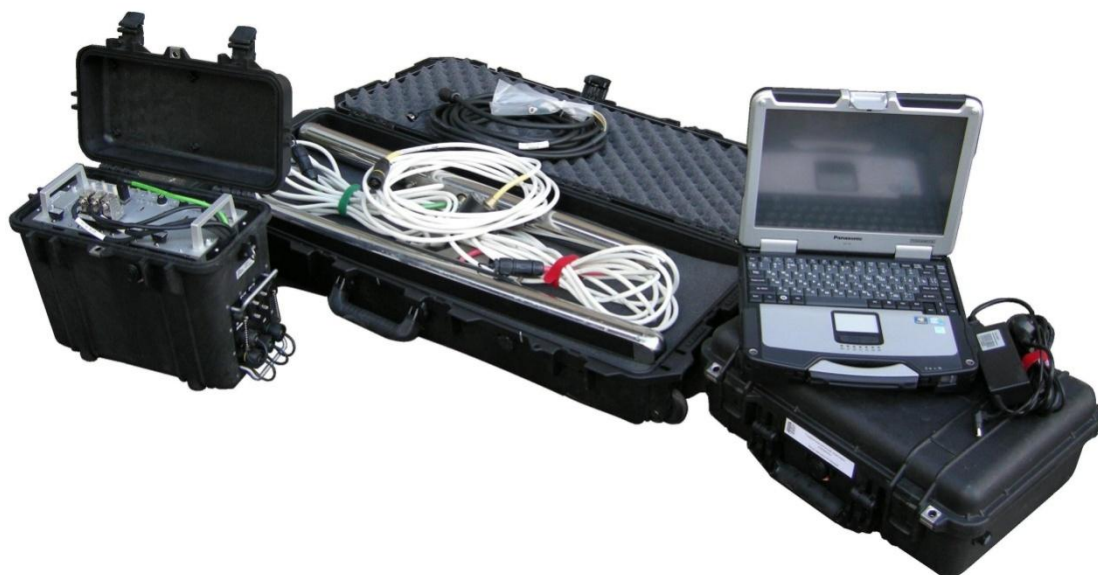
Fig. 3. Mobile side scan sonar complex “Neman GBOE” (general view).
