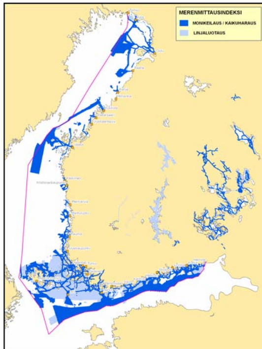
Fig 1. Status of hydrographic survey data. Dark Blue: Multibeam Light blue: Single beam
