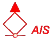
Figure 1 - Portrayal of a virtual AIS AtoN - starboard lateral mark.
