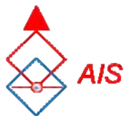
Figure 2 - Blue AIS diamond symbol on top of the ‘ENC symbol’
