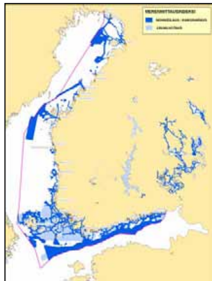
Fig 3. Status of modern hydrographic survey data at end of 2007. Dark Blue: Multibeam Light blue: Single beam
