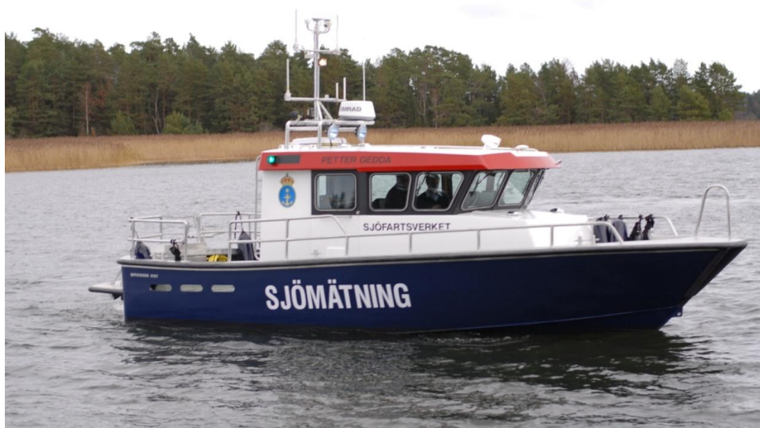
Fig 4 PETTER GEDDA, a 8.5m boat built for near shore and port jobs. Equipped with RESON 7125 multibeam echo sounder.
