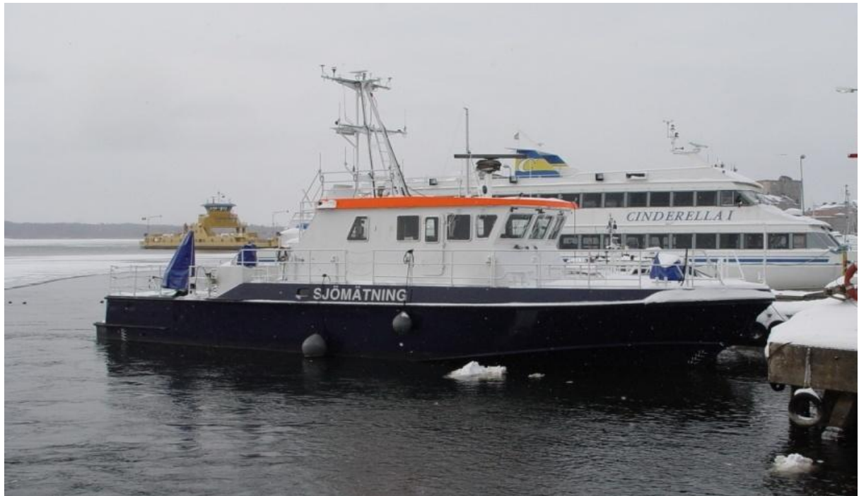
Fig 5 JOHAN MÅNSSON a 20m boat equipped with RESON 7125 multi-beam echo sounder for work in the Swedish archipelago. The crew will be 3-4 persons with two work places for post processing.
