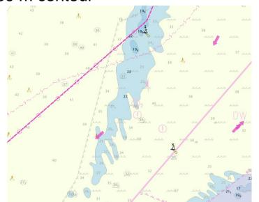
ECDIS With Band 6 cell – defaults to 22 m contour in area of cell
