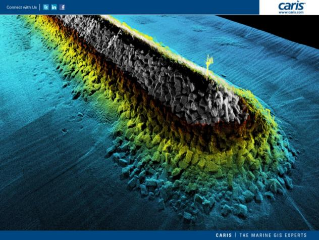
Also after port construction maintenance surveys are needed, for example to inspect the state of quays, as is seen here, or to make an assessment of the port areas that need to be dredged. The underwater part of the quay shown here is based on data processed in CARIS HIPS and SIPS.
