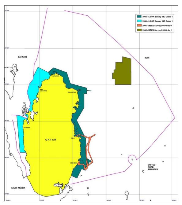
Adequately surveyed are has been increased with two surveys concluded by the USA Naval Oceanographic Office in 2005, and French Hydrographic and Oceanographic Service in 2006.
