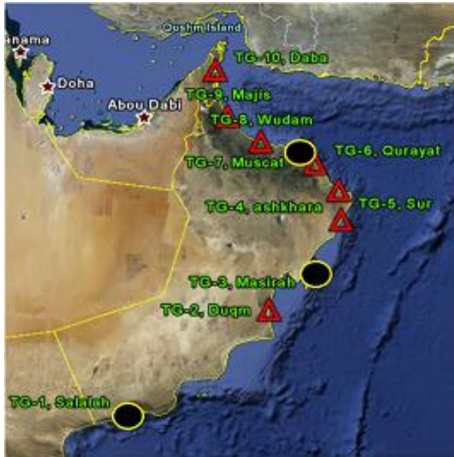
Figure-1. Sea level network in Oman, consists of 3 current stations (black circles) and new stations (red triangles).
