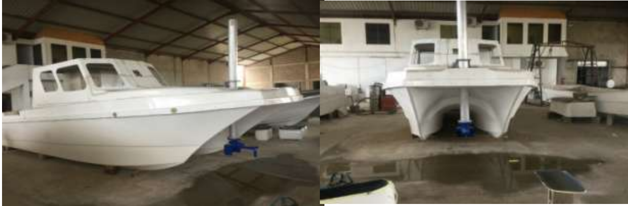
New survey work boat under construction
