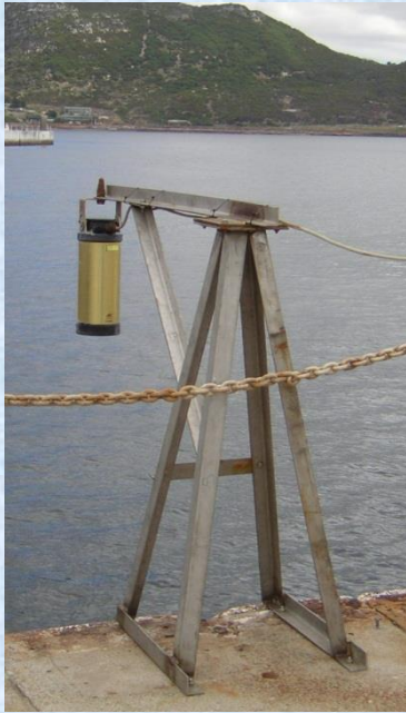
Acoustic Tide Gauge continuously recording tidal level
