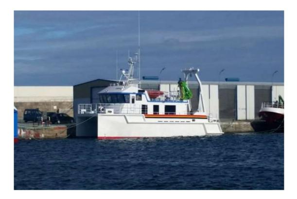
HYDROGRAPHIC COASTAL BOAT: Used for conducting studies, bacthymmetric surveys at the Angolan coast level to provide data that are used to define navigation channels, update nautical documents.
