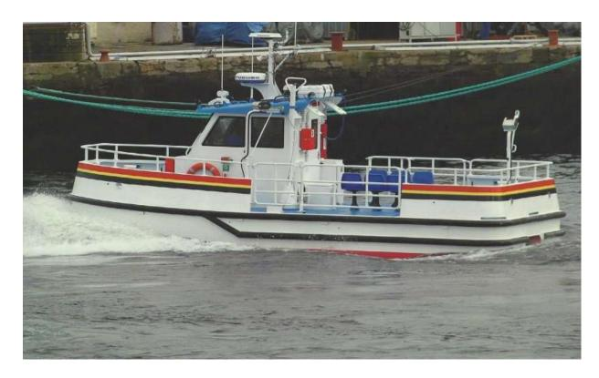
**PORT HYDROGRAPHIC BOAT**: It has as purpose or objective to carry out internal survey /study at the level of the Ports, in order to get data that are used for definition of navigation channels, updating of nautical documents.
