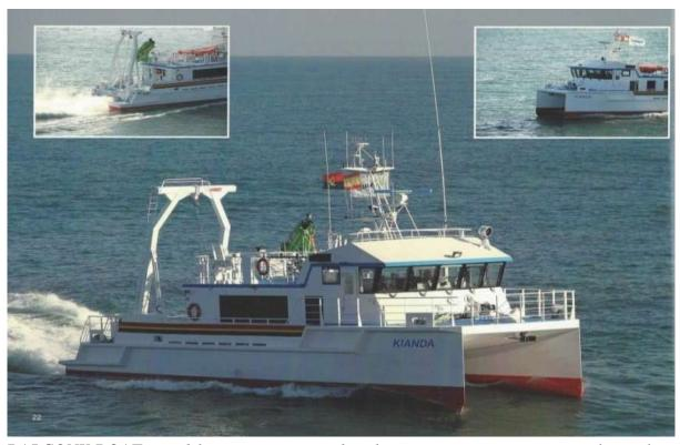
**BALCONY BOAT**: Used for carrying out studies that serve as support in nautical signaling, as well as the implantation of buoys.
