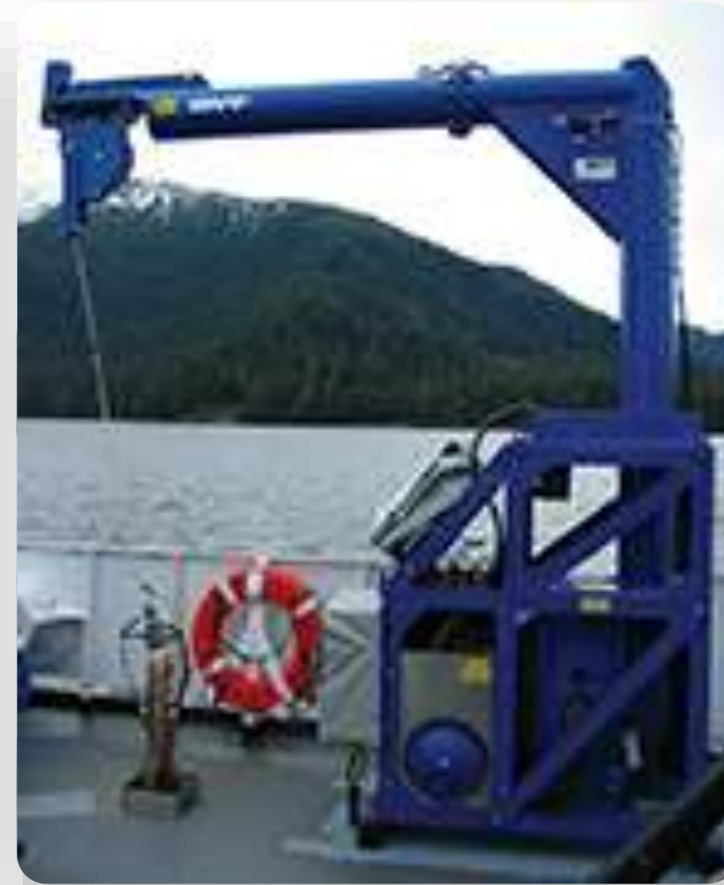
MVP200 Profiles to 200m WD at 12 knots, and 310m at 6 knots
