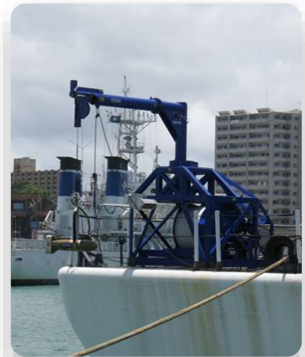
MVP300 Profiles to 300m WD at 12 knots, and 1250m at 6 knots
