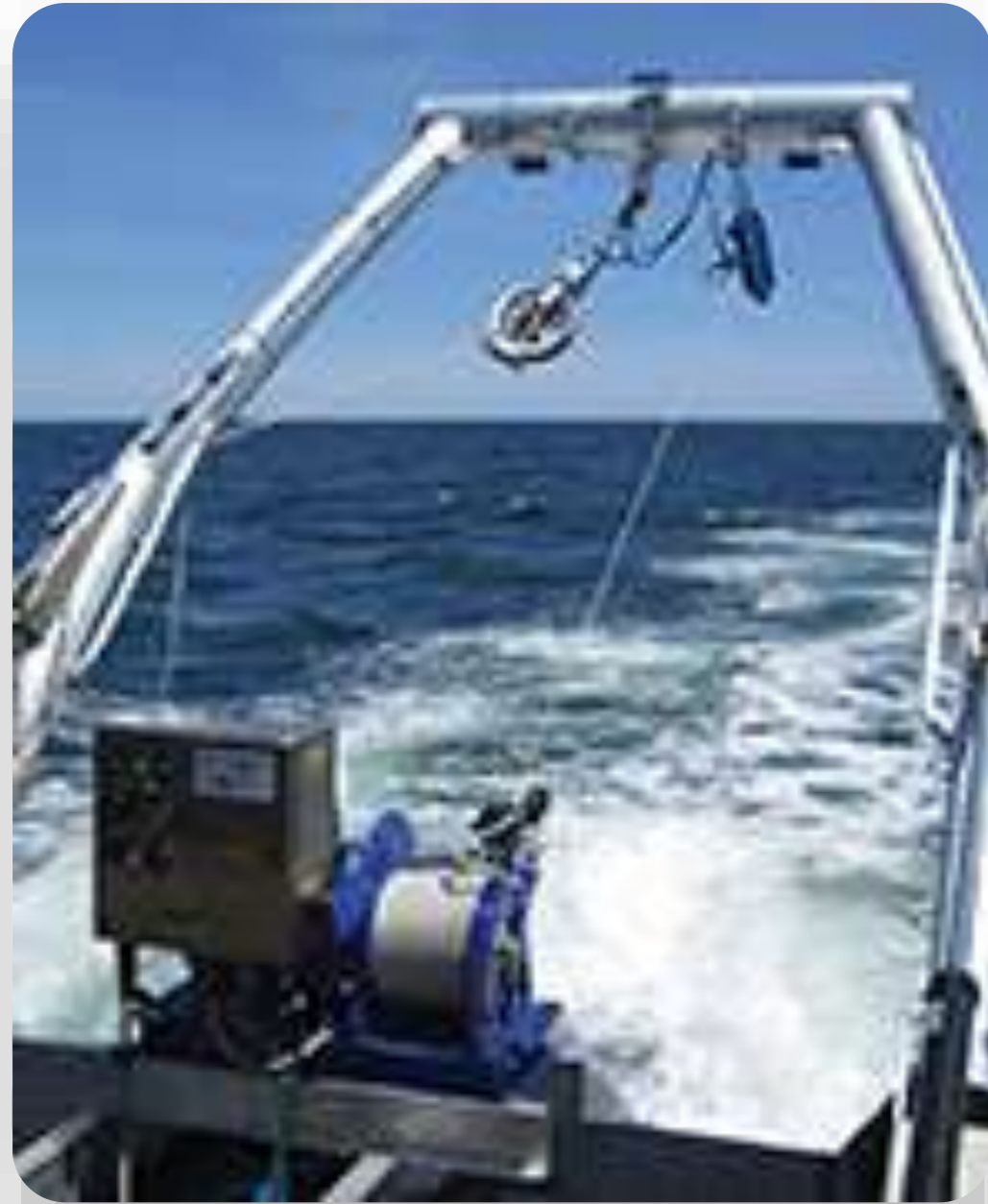
MVP30/350* Profiles to 30m WD at 12 knots, and 155m* at 6 knots
