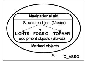
If it is required to encode the name of the navigational aid, it must be done using the attribute OBJNAM (and possibly the attribute NOBJNM) on the master object. The name should not be repeated for the slave objects. If the name is painted on the structure, it must be encoded with the same spelling in OBJNAM if it is based on the Latin alphabet. If the name is not based on the Latin alphabet, it must be encoded on NOBJNM, and transliterated for encoding on OBJNAM.
