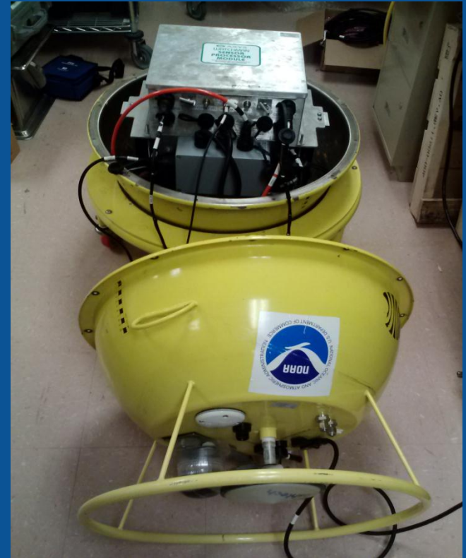
AXYS Hydrolevel Water Elevation Monitoring Buoy
