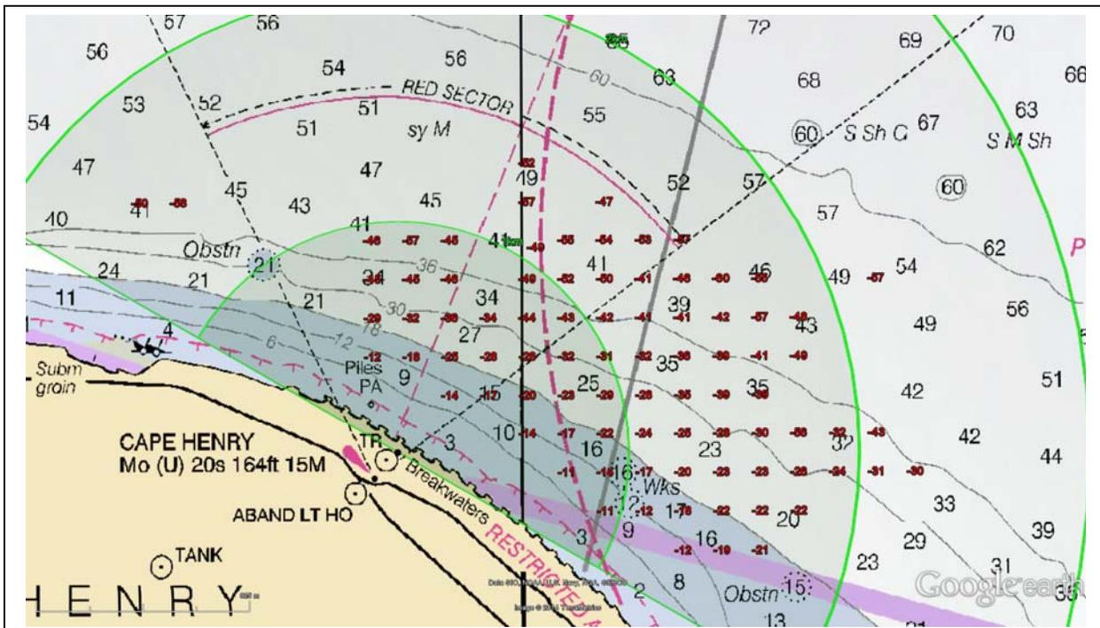
**Figure 18.** Cape Henry Radar Bathymetry. This is NOAA Chart #12254 with the radar bathymetry overlaid. The red numbers are the bathymetric radar retrievals from the 336m x 336m tiles with 50% overlap. The green rings indicate ranges of 1 km, 2 km and 3 km
