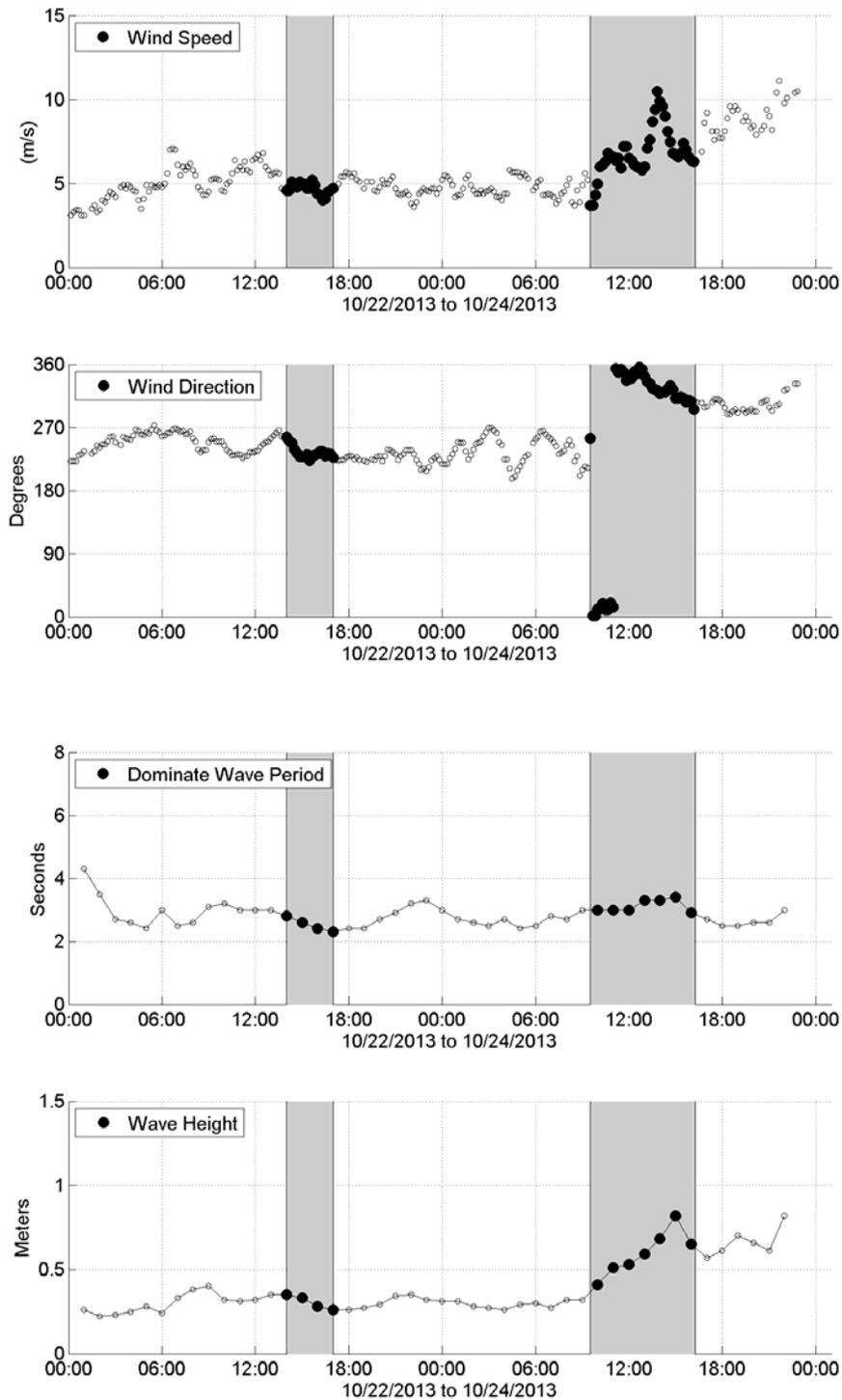
**Figure 5.** Wind and wave data during CBBT collections. The data was obtained from NOAA buoy 44064 located east of the radar. The grey areas indicate the time of collections.
