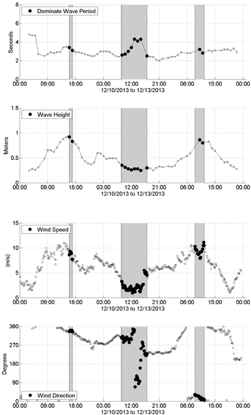
**Figure 6.** Wind and wave data during Cape Henry collections. The data was obtained from NOAA buoy 44064 located east of the radar. The grey areas indicate the time of collections.
