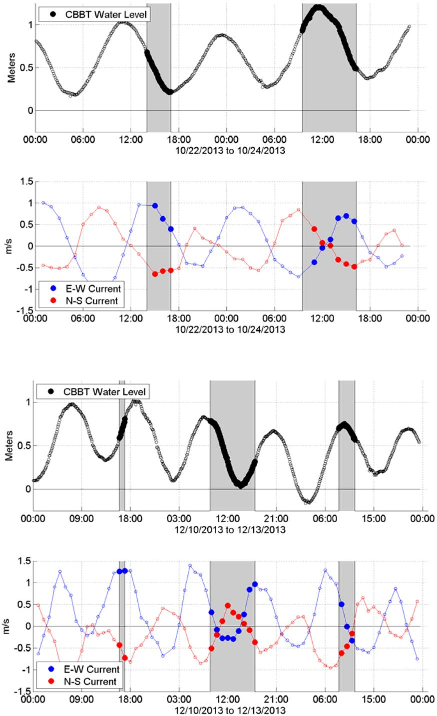
**Figure 7.** Water level and currents during CBBT and Cape Henry collections. The current data was obtained from NOAA buoy 44064 located east of the radar and water level is from the tide gage located at Island One (Station ID 8638863). The grey areas indicate the time of collections.
