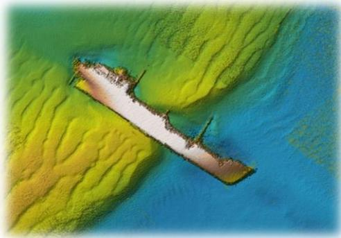
*A wreck detected by side scan sonar*
