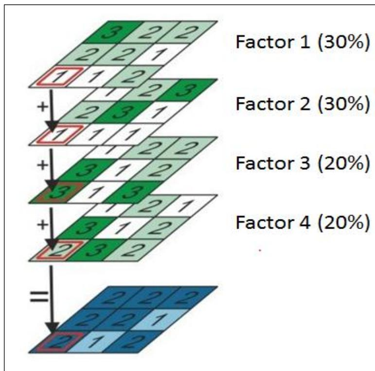
Figure 3: Weighted overlay analysis methodology.
