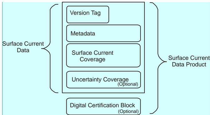
Figure 3 - Overview of Structure of Surface Current Data Product
