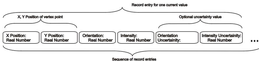
Figure B-6 - S111 Surface Current Point Set Coverage Record Structure with the optional uncertainty value(s).
