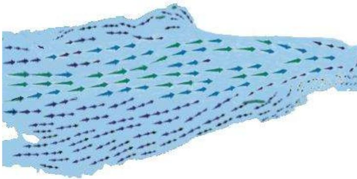
Figure 2 - An Example of a Point Set Coverage of Surface Currents
